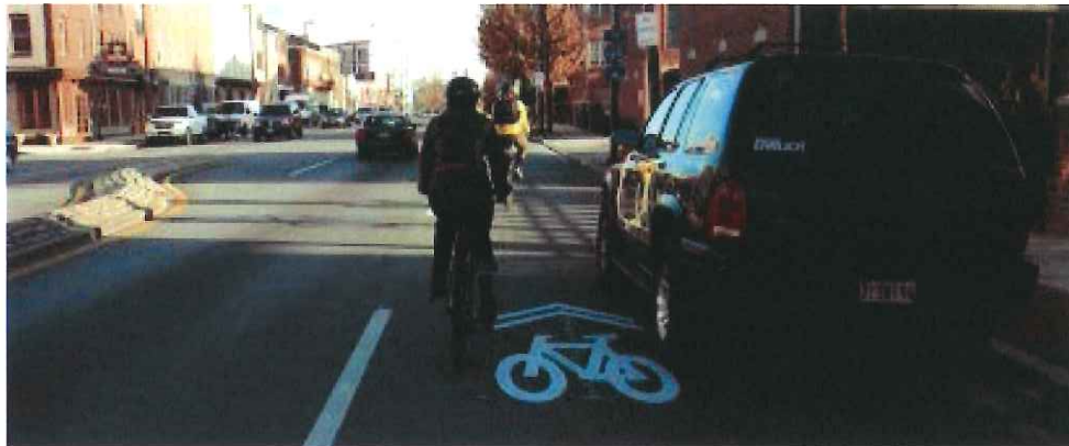
Figure 202: Shared Lane Marking Placement while Off-Peak Parking Allowed 15
