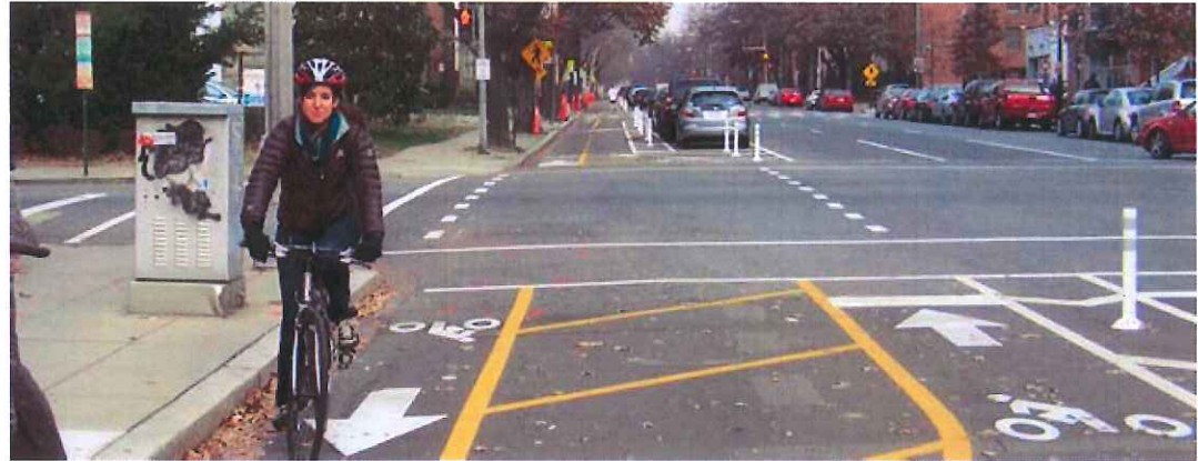
Figure 13: Example of Bollards to Buffer Bicycle Lanes 8
