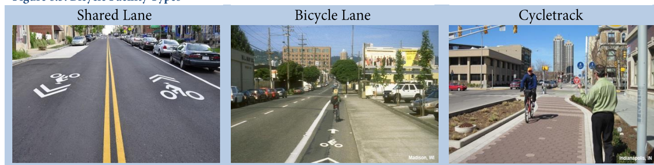
Figure 6.5: Bicycle Facility Types
